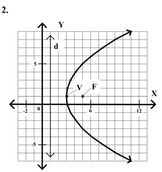
2. This is an example of the second type of parabola (axis horizontal). Since the vertex is (3, 1), h = 3 and k = 1.
